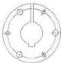
Bushings JA to J inclusive Drilled for Standard or Reverse Mounting
